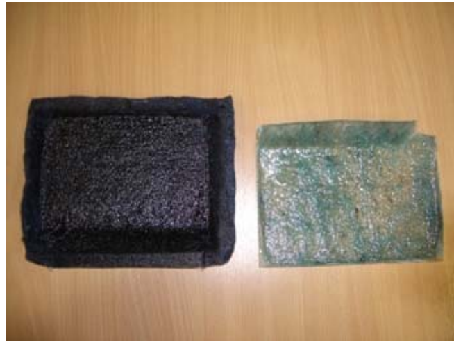
Figure 9: Formed Composite Materials Reinforced with Clothing Fibre Waste
